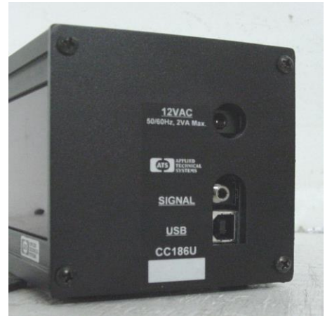
Power and Signal Jacks
